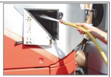
Raise the dirt hopper approx. 50 % so that the water and dirt can be tipped out. Clean the entire dirt hopper from the inside.
